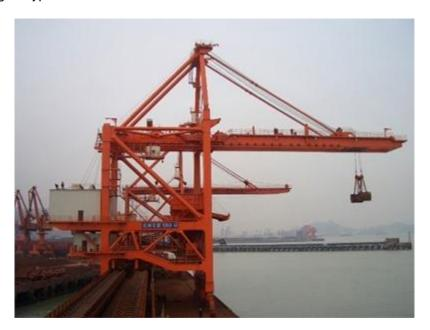
Figure 6-1 Grab type bulk unloader
