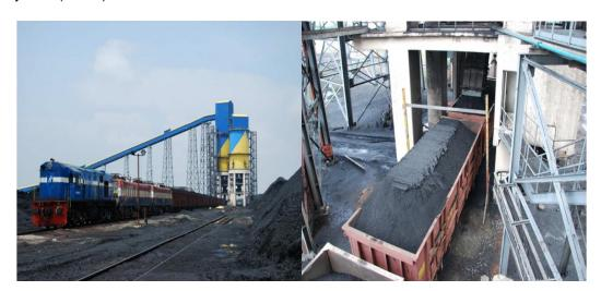
Figure 6-3 Rapid Rail Loading System
