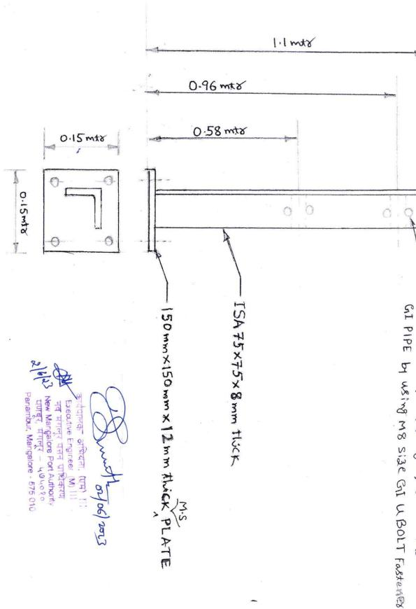
4 NOS holes for fixing of 32 mm NB
