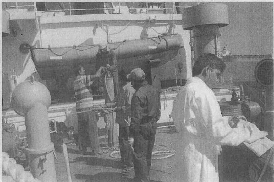
4. Application of pressure through nitrogen cylinder for injection of tracer material
